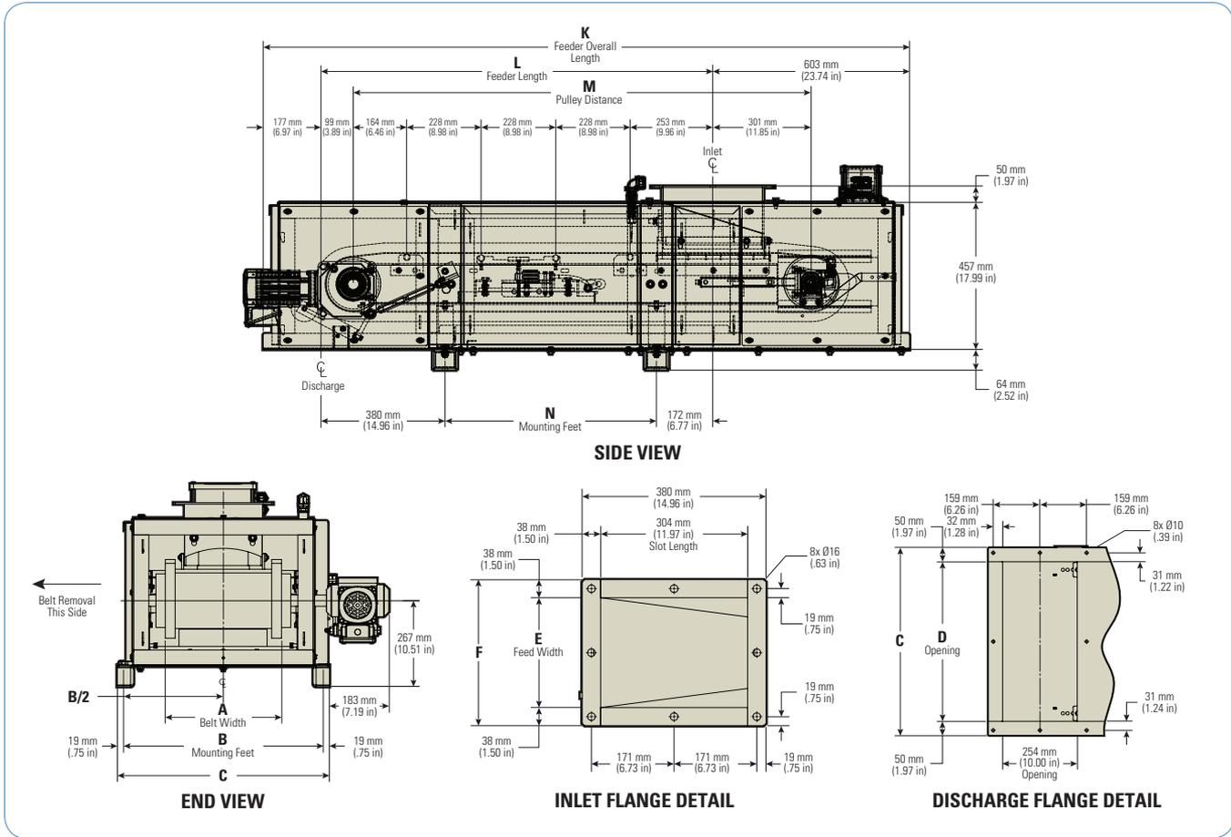
Ramsey Model 90-150 Low Capacity Weighbelt Feeder — Variable Dimensions
