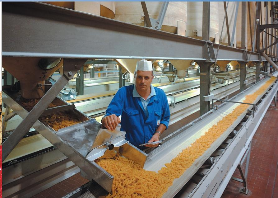
**Cantilevered frame and quick release take-up for easy belt removal**
